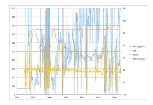
152. Another instance in the following plot, where the reduction in SCR effectiveness begins to reduce at 2,900 seconds. The SCR effectiveness reduces from well over 90% to approximately 50%, just as before, with a composite NOx emission rate of 428 mg/mile. Prior to the reduction in urea injection, the emission rate is 58 mg/mile, well below the standard. After the reduction in urea injection, the emission rate increases to 586 mg/mile.
