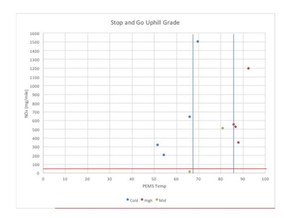
137. For steady highway driving, grades between 0.5% and 3.5% were tested. Emission levels were measured as high as 4,558 mg/mile, with an average of 942 mg/mile. These are extraordinarily high numbers given the relatively low road grade. The SCR effectiveness drops from 88% in cases where the vehicle meets the standard on flat roads during highway driving to 54%. Similarly, the EGR rates drops from 47% to 32% for the flat road and uphill grade conditions, respectively.
