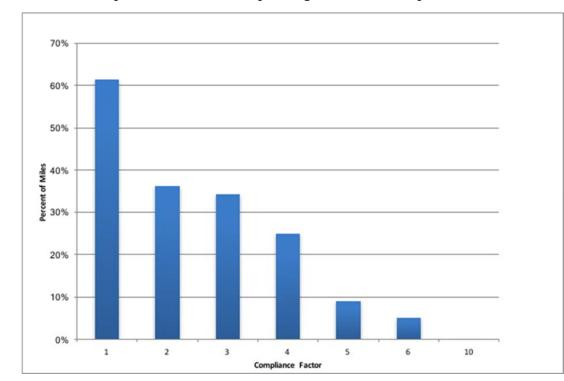
144. The vehicle spends 61% of its time above the standard. That means only 39% of the miles traveled in stop-and-go conditions actually met the standard. The vehicle spends fully 25% of the time more than four times the emission standard.
