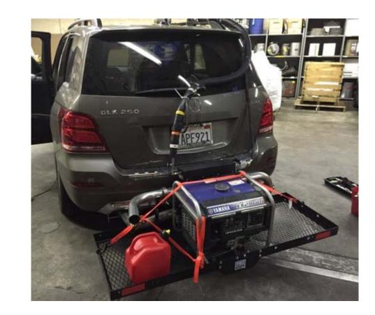
85. The stop-and-go emissions were found to be 208 mg/mile on average over all tests conducted, or 4.2 times the standard of 50 mg/mile. Maximum emissions in stop-and-go conditions were found to be 1,725 mg/mile, a condition where the EGR and SCR systems had been completely shut off. That is 34.5 times the standard.
