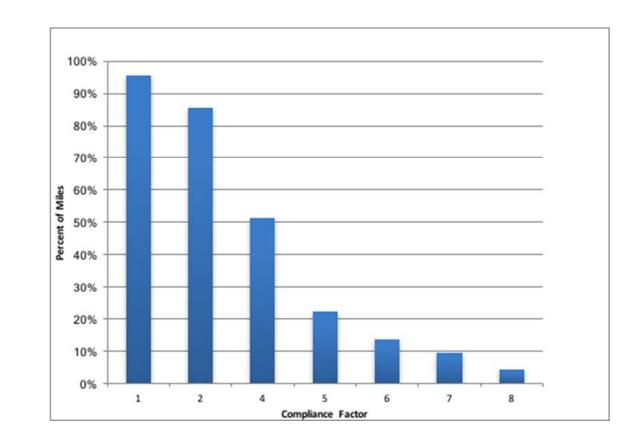
148. The vehicle spends 96% of the miles traveled above the standard, leaving only 4% of the vehicle miles traveled (VMT) having met the standard. The vehicle spends 51% of its VMT at four times the standard of above, and 4% at eight times the standard or above.
